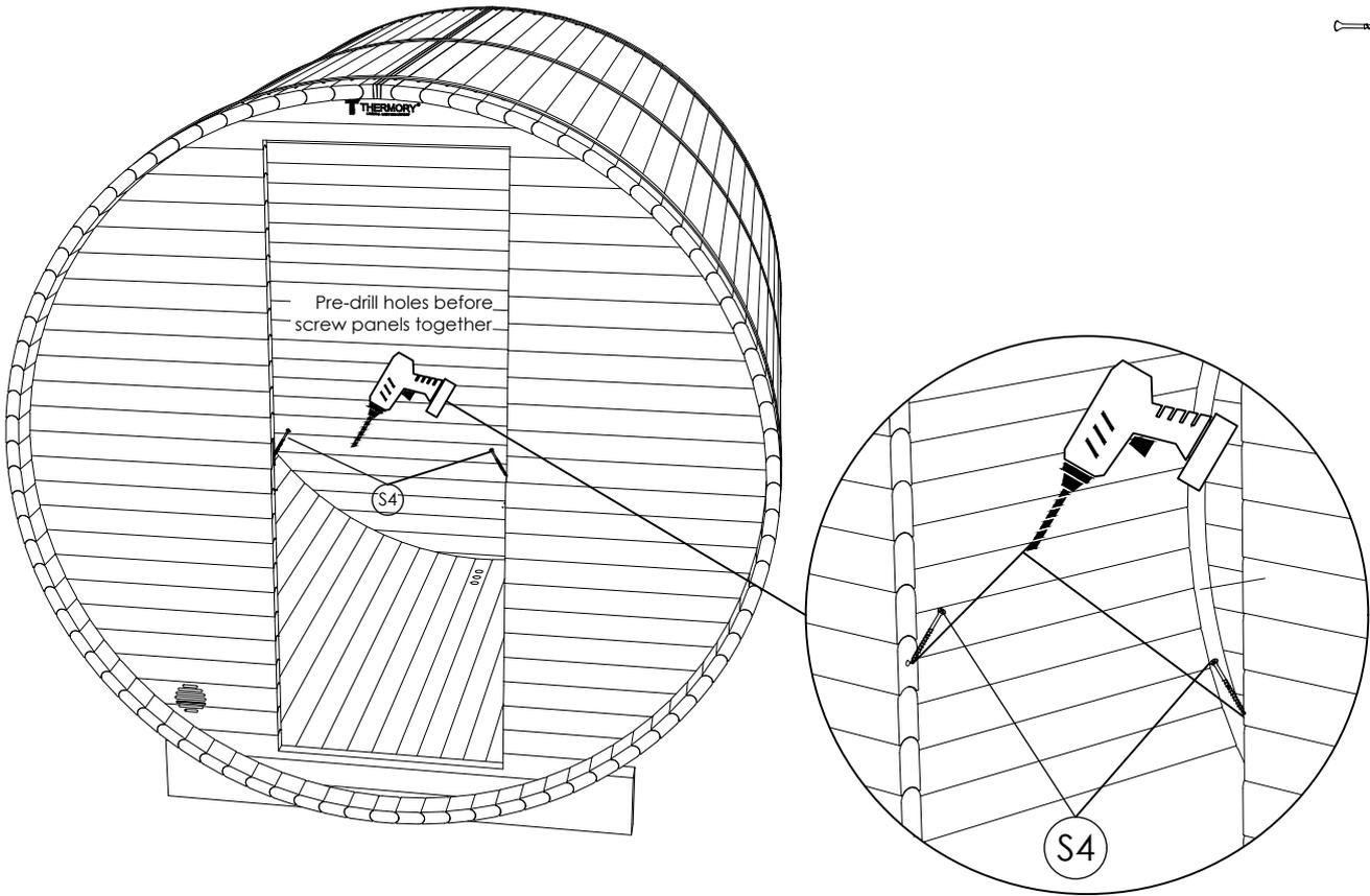
**STEP 14:** Install the doors (F2). Put the doors on threshold and lay in frame about in the middle. Fix doors with clamps or another person should hold the door.
