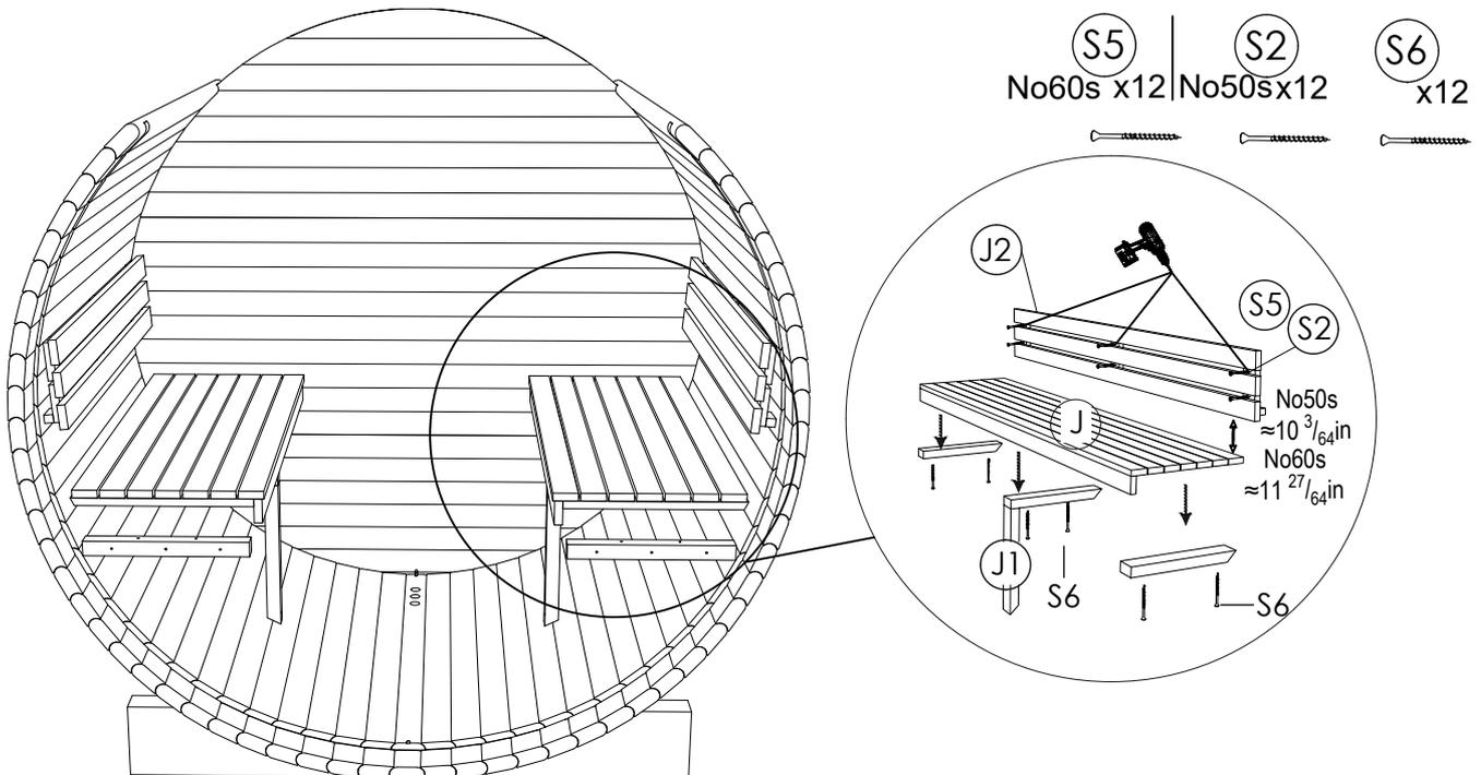
**STEP 19:** Place floor duckboards (L) to the both sides upwards and place fixing blocks next to the flooring cross boards. Pre-drill holes before fix with screws, install fixing blocks (L1) using screw(S2)No50s or (S5)No60s.
