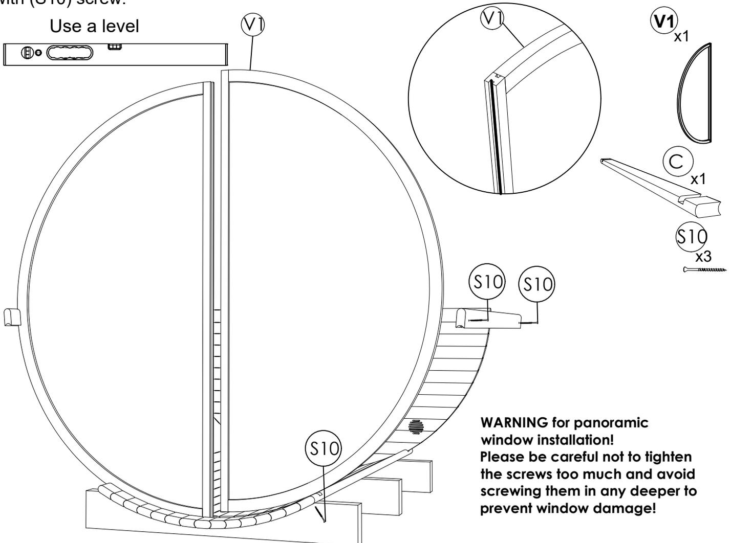
**STEP 5:** Fix Assembly tape with five screws (S12) to fix both panels together. Continue placing body staves (C) tightly on both sides of the sauna using rubber mallet, and fixing body staves with screws (S10), two screws for each staff.
