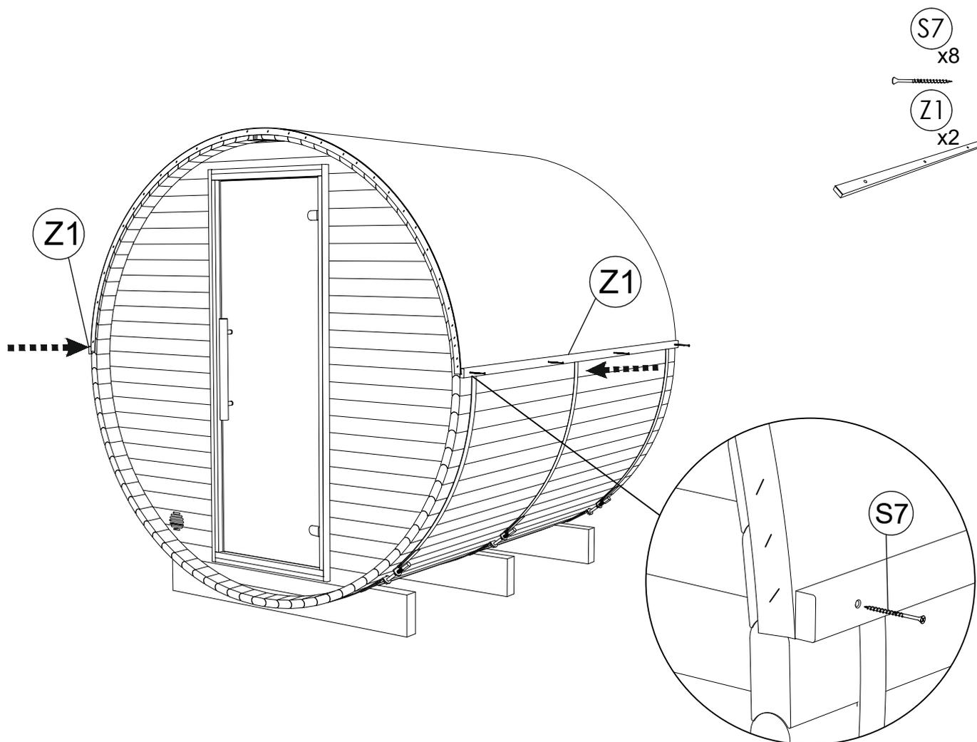
**STEP 24:** Install front and rear decorative roof finishing boards (W), fixing by screws (S7). Start with a center board placing it at the top of the middle of the sauna, approx.  $\frac{50}{64}$ in above roof or  $\frac{13}{64}$ in under the roof. Then fix next boards right next to previous board.
