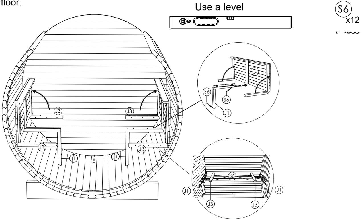
**STEP 18:** Pre-drill holes before fix backrest with screws, install backrests (J2) using screw (S2). Fix sauna bench (J) to wall mounts and support leg using (S6) screws.
