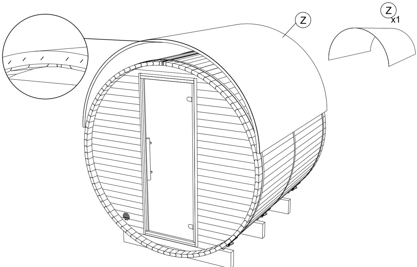
**STEP 23:** Fix with wooden slats (Z1) with screws (S7) on the rain jacket bottom. The number of screws may vary depending on the sauna model.
