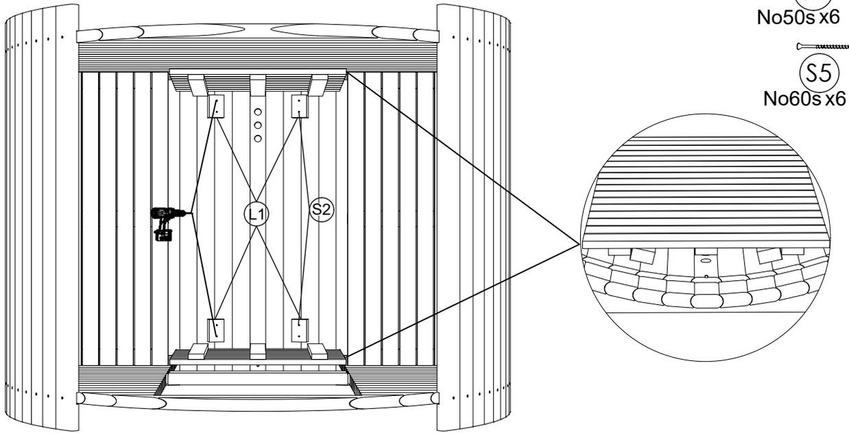
**STEP 20:** Pre-drill holes before fix with screws, install fixing blocks (L1) under floor duckboard using screw (S2) No50s or (S5) No60s. Place floor duckboards (L) on the floor and fix fixing blocks next to both flooring crossboards.
