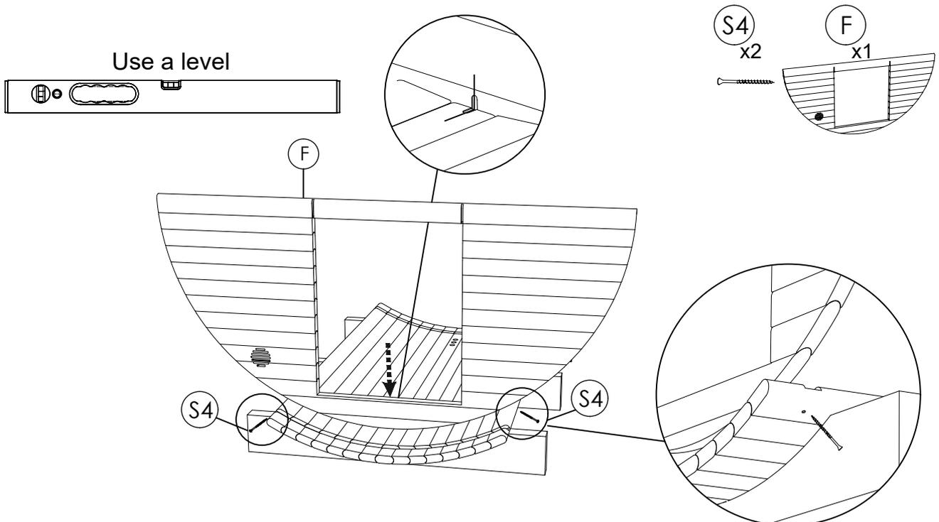
**STEP 1:** Apply silicone evenly in the groove of the rear panel (V1) for wood spacer bar (V1-F).
