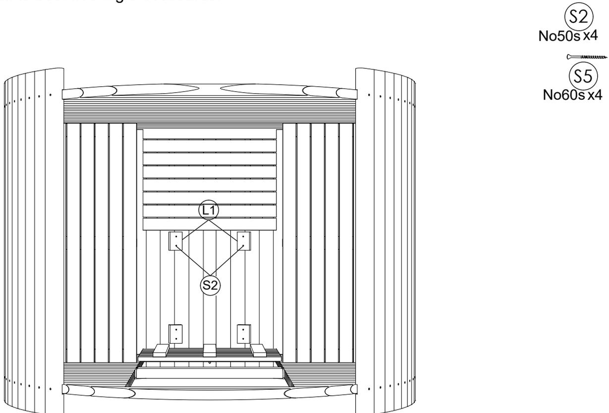
**STEP 21:** Pre-drill holes before fix stave with screws, install interior roof trim (O) in sauna with (S5) screws.
