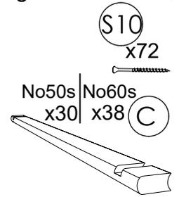
**STEP 10:** To finish the roof top joint, don't screw about last 2-3 boards (C) to each side, use roof finishing item (H). Different thickness filling pieces (H1) are provided to completely fill the gap. Once necessary parts are in, fix last boards with screws.
